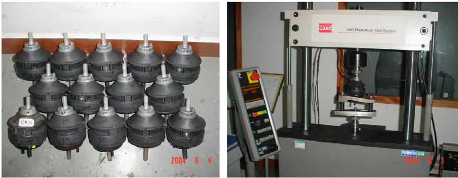
Fig. 3. Some test samples (left) and the test rig (right).
